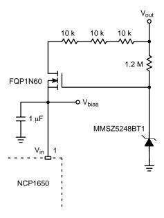
Figure 1. Start-Up Circuit Schematic
